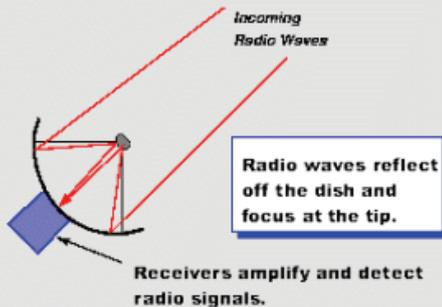
Radio telescopes are used to study naturally occurring radio emission from stars, galaxies, quasars, and other astronomical objects between 30MHz and 300GHz. At wavelengths longer than about 1.5 GHz, irregularities in the ionosphere distort incoming signals. This causes a phenomenon known as scintillation, (twinkling). The absorption of cosmic radio waves by the ionosphere becomes more important as wavelength increases. At frequencies higher than 30Mhz, the ionosphere becomes
